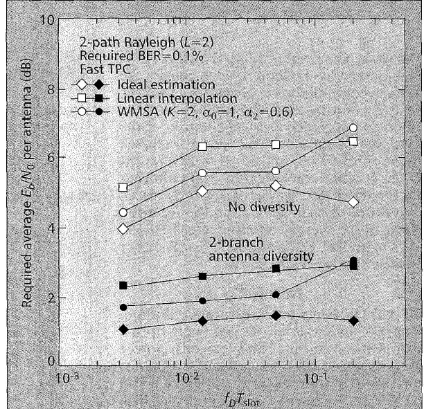
**■ Figure 9.** Measured required  $E_b/N_0$  with fast TPC.
