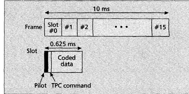
■ Figure 1. Frame structure using time-multiplexed pilot.
