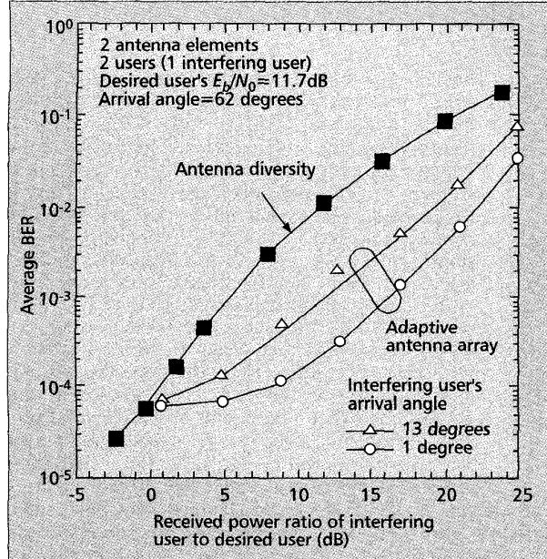
**Figure 21.** Measured average BER as a function of received power ratio of interfering user to desired user.
