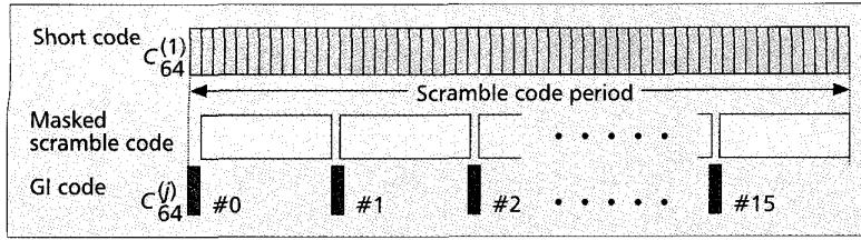
■ Figure 3. Scramble code masking timing and GI code transmission.
