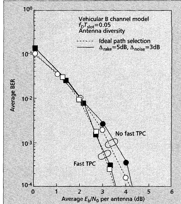
**Figure 22.** Average BER performances with MF-based Rake receiver.
