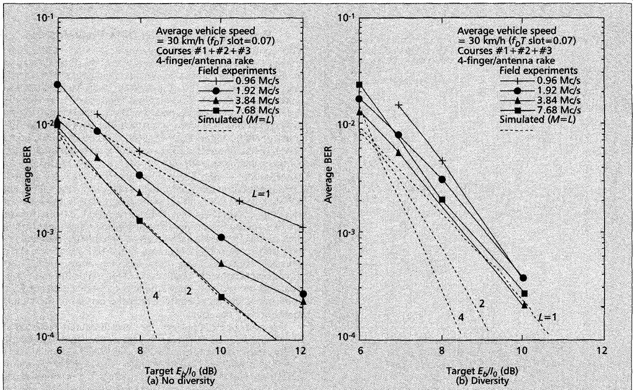
■ Figure 15. Comparison of average BER performance with different chip rates.
