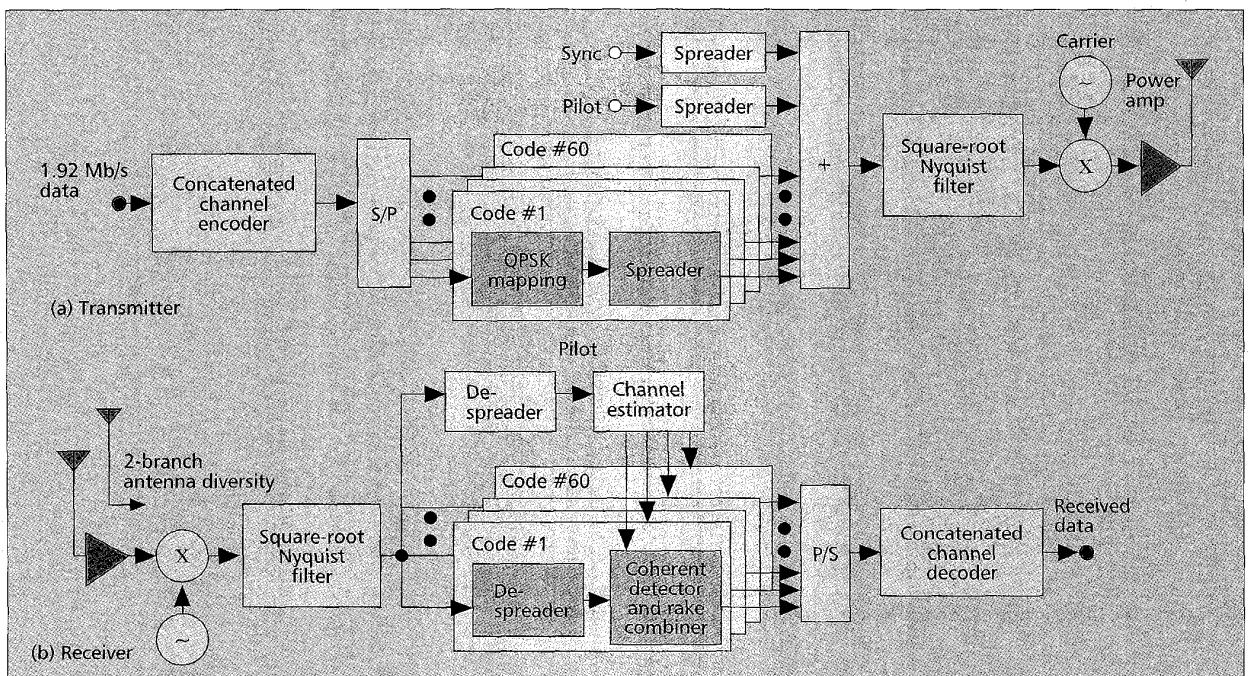
■ Figure 16. Experimental 1.92 Mb/s transmitter and receiver.
