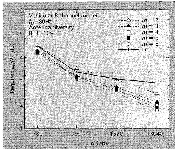
■ Figure 24. Turbo coding effect on required  $E_b/N_0$ .
