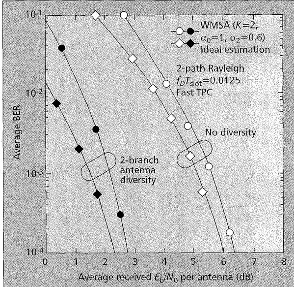
**■ Figure 8.** BER performance with WMSA coherent Rake receiver.
