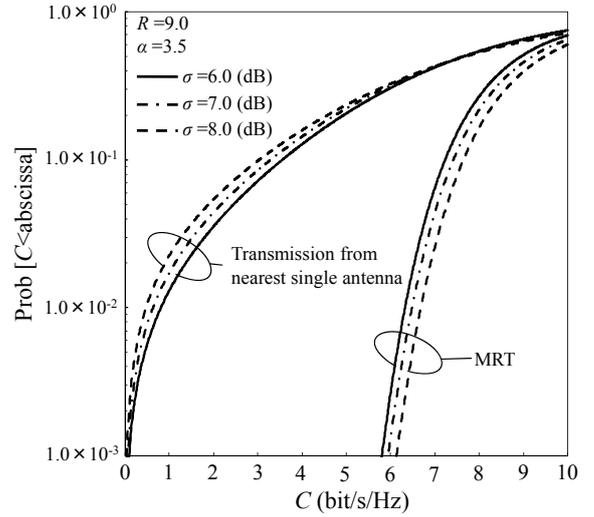
Fig.6 Impact of shadowing loss standard deviation  $\sigma$ .
