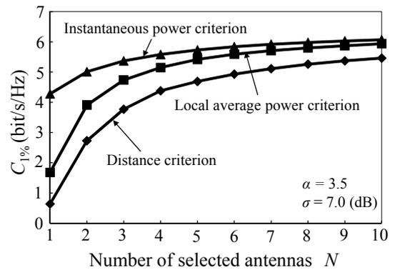
Fig.9 Comparison of three antenna selection criteria.
