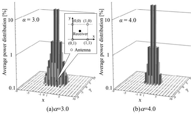
Fig.5 Impact of  $\alpha$  on antenna power distribution.
