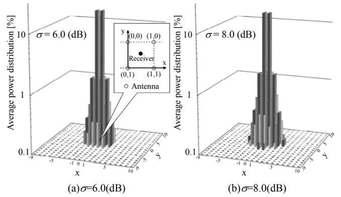
Fig.7 Impact of  $\sigma$  on antenna power distribution.
