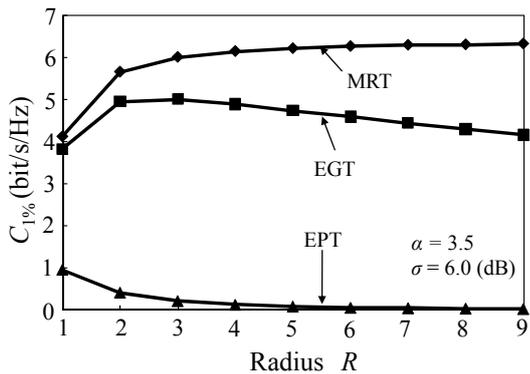
Fig.3 Comparison of MRT, EGT and EPT.
