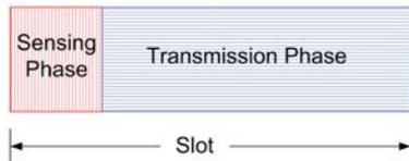
Figure 1: The slot structure of the secondary networks.
