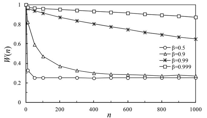
Figure 6. Autocorrelation  $W(n)$  of channel distribution pattern.
