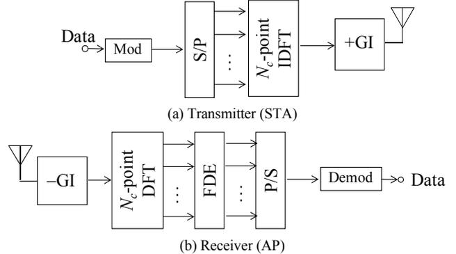
Figure 2. Uplink transmission system model of OFDM.
