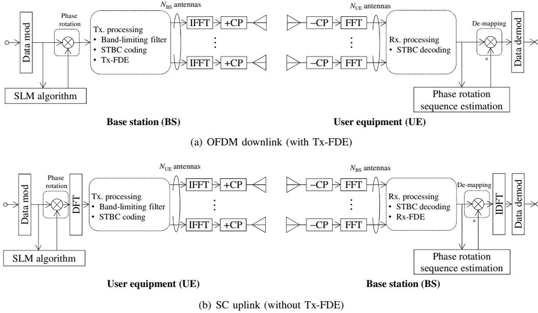
Fig. 1. Transceiver model with STBC-TD and blind SLM.
