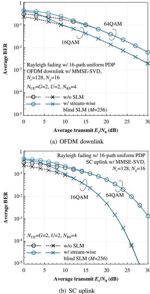
Fig. 4. BER performance of MMSE-SVD with blind SLM.
