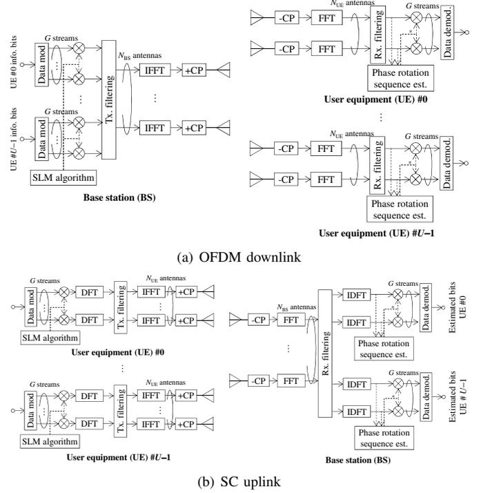
Fig. 2. MMSE-SVD system models with blind SLM.
