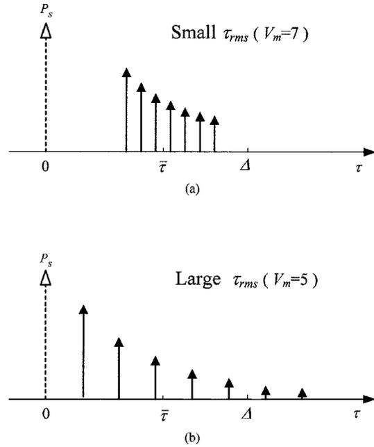
Fig. 3. Illustration highlighting the effect of varying  $\tau_{\text{rms}}$  on the relative position of the power profiles against the guard interval length  $\Delta$ , with a constant average delay  $\bar{\tau}$ .
