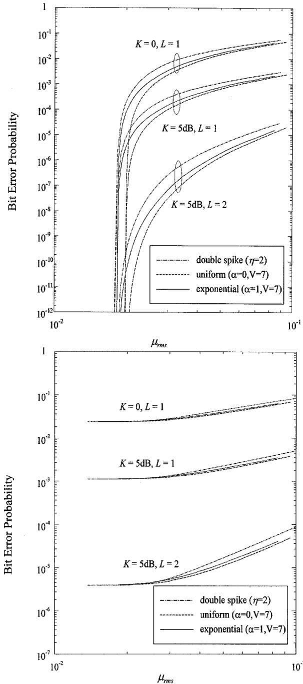
Fig. 6. (a) Average BER of OFDM-QDPSK system in frequency selective Rayleigh and Rician fading with  $M = 4, f_D T_b = 0, N = 32, \Delta/T_b = 0.15, \bar{\tau} = 0.8\Delta$ . (b) Average BER of OFDM-QDPSK system in frequency selective Rayleigh and Rician fading with  $M = 4, f_D T_b = 0.05, N = 32, \Delta/T_b = 0.15, \bar{\tau} = 0.8\Delta$ .
