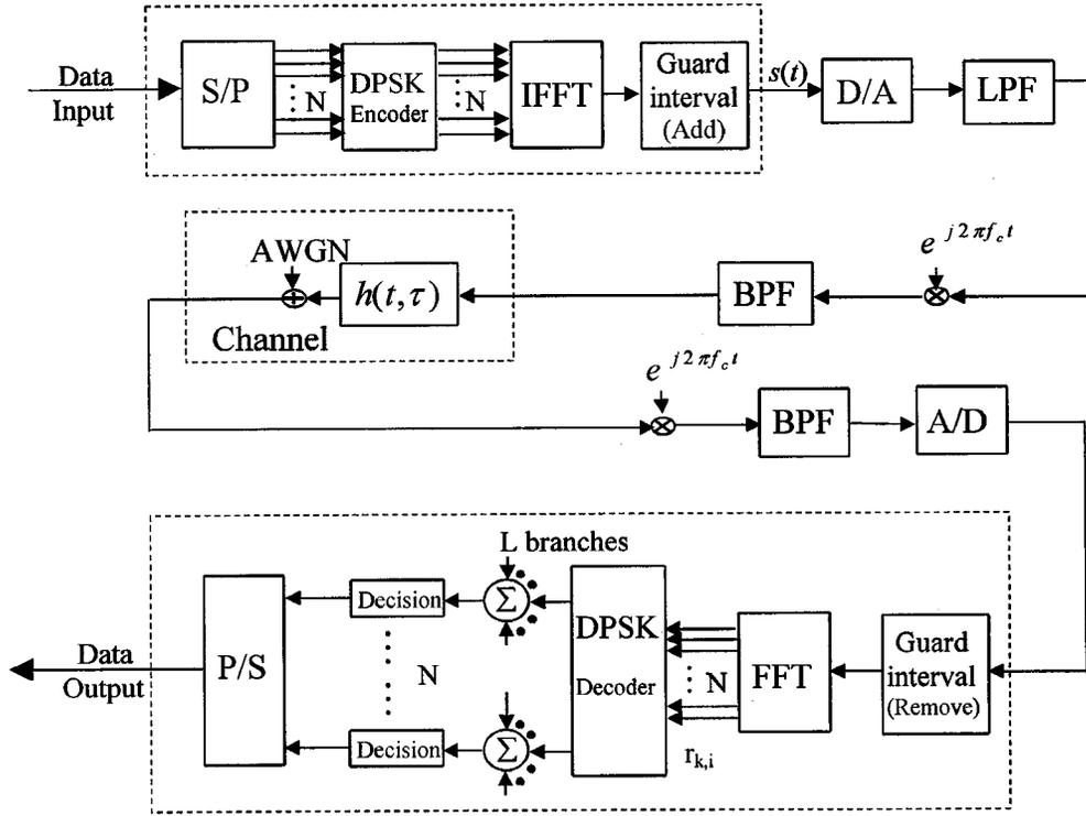
Fig. 1. Block diagram of the OFDM-MDPSK system.
