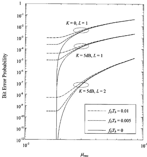
Fig. 5. Average BER of OFDM-QDPSK system in frequency selective Rayleigh and Rician fading with one-sided exponential delay profile with  $\alpha = 1, V = 7$ , and  $M = 4, N = 32, \Delta/T_b = 0.15, \bar{\tau} = 0.8\Delta$ .
