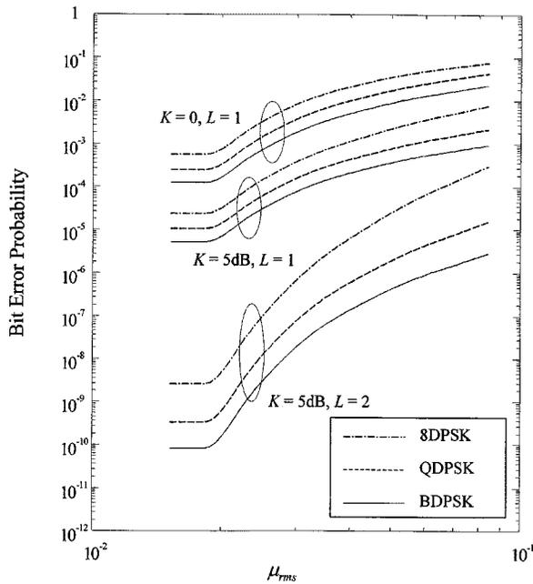
Fig. 4. Average BER of OFDM-MDPSK system in frequency selective Rayleigh and Rician fading with one-sided exponential delay profile with  $\alpha = 1, V = 7$ , and  $f_D T_b = 0.05, N = 32, \Delta/T_b = 0.15, \bar{\tau} = 0.8\Delta$ .
