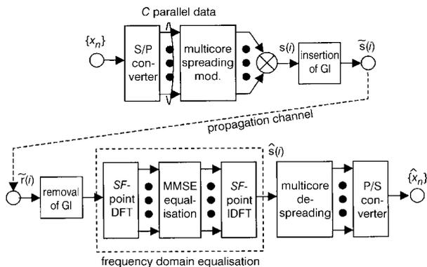
Fig. 1 Multicore DS-CDMA transmission model
