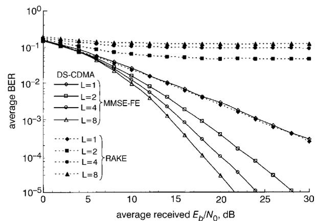
Fig. 2 Comparison of DS-CDMA with MMSE-FE and with RAKE combining
