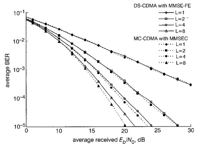
**Fig. 3** Comparison of DS-CDMA with MMSE-FE and MC-CDMA with MMSEC
