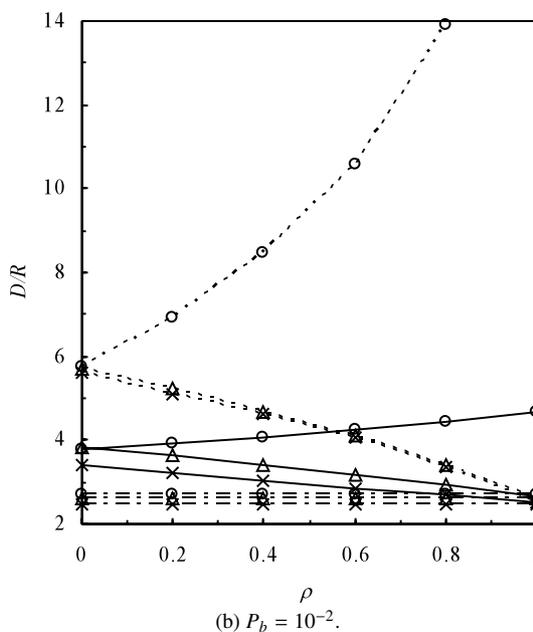
Fig. 4 Normalized frequency reuse distance as a function of shadowing correlation  $\rho$  for uplink ( $\chi=10$  dB,  $Q_0=0.1$  and  $M=2$ ).
