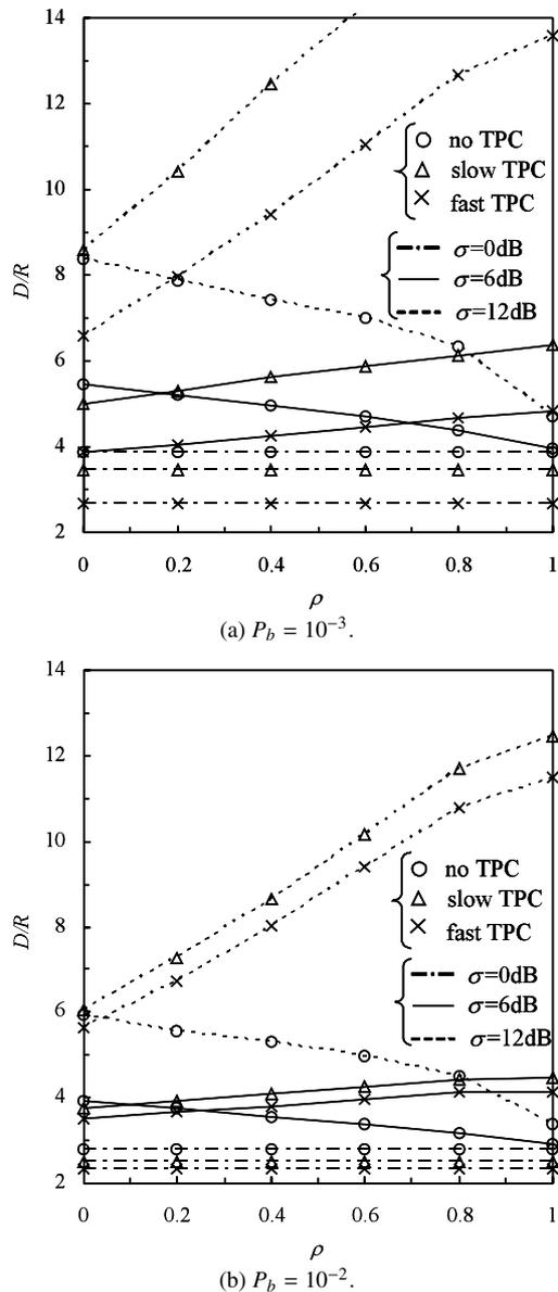
**Fig. 5** Normalized frequency reuse distance as a function of shadowing correlation  $\rho$  for downlink ( $\chi=10$  dB,  $Q_0=0.1$  and  $M=2$ ).
