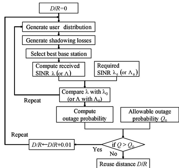
**Fig. 3** Flow chart for computer simulation.
