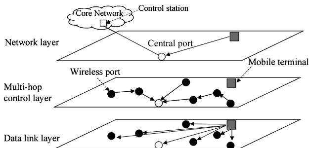
Fig. 2 Layer structure of wireless multi-hop VCN.
