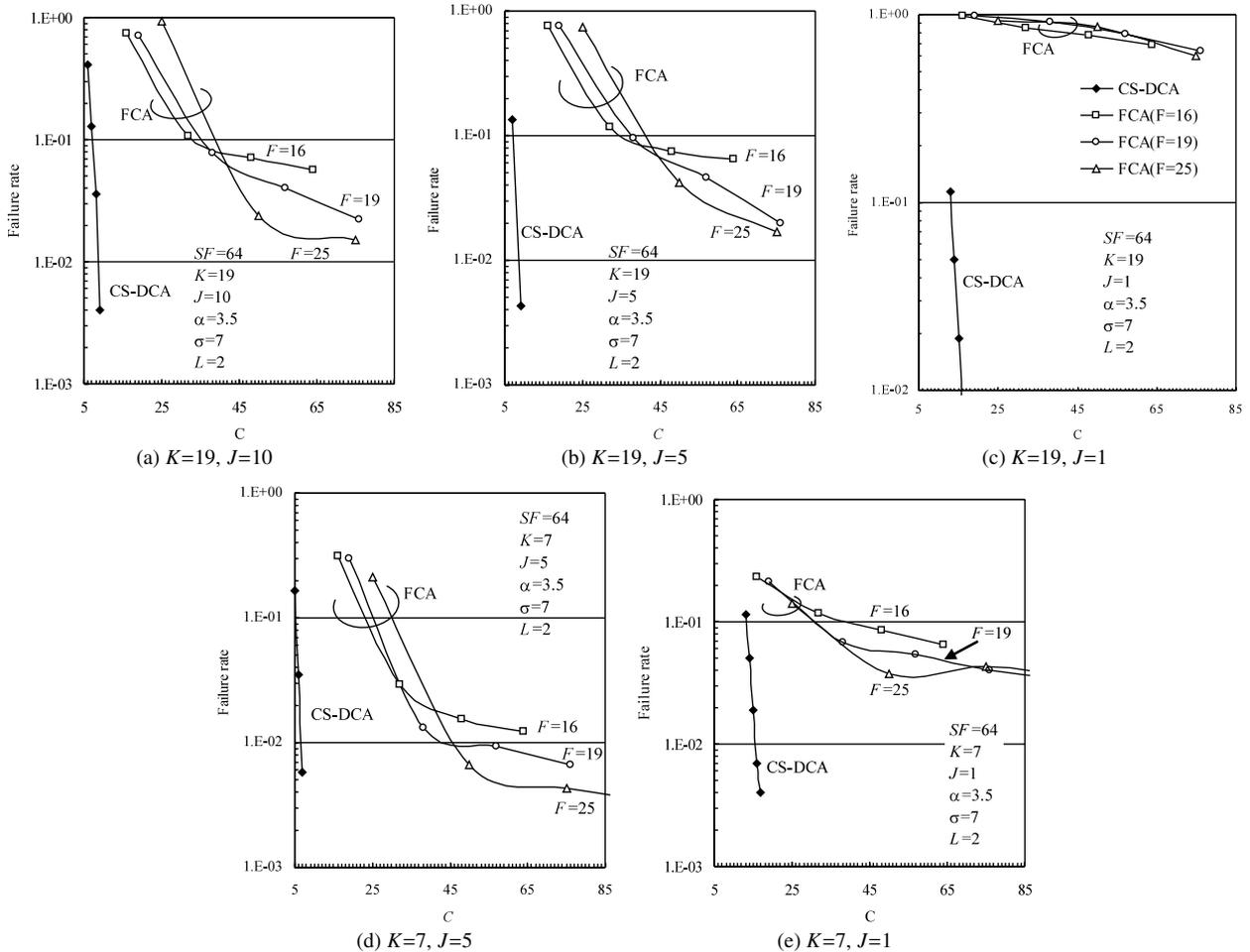
Fig. 5 Comparison of CS-DCA and FCA.
