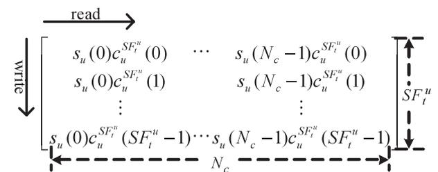
Fig. 2 Chip-interleaving.
