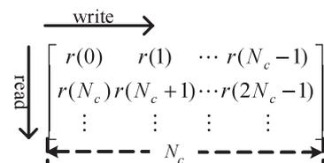
Fig. 4 Chip-deinterleaving.
