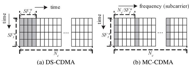
Fig. 3 2D OVFS spreading and chip-interleaving
