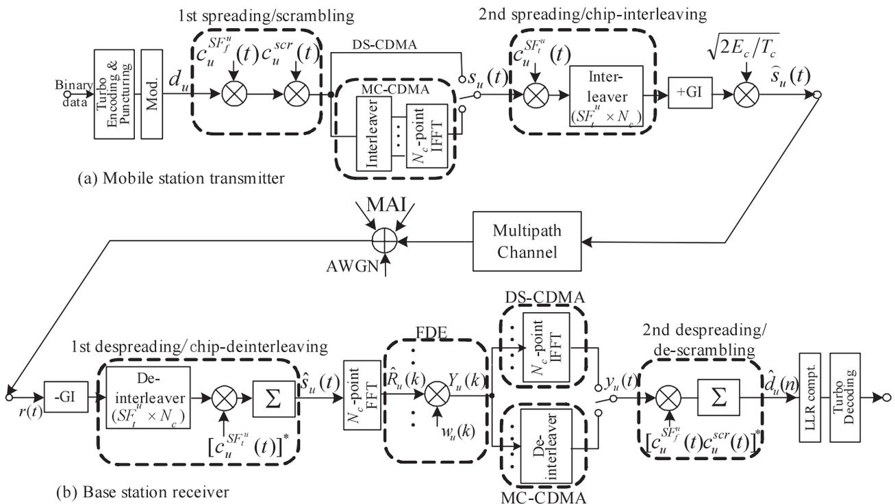
Fig. 1 Uplink transmitter/receiver structure.
