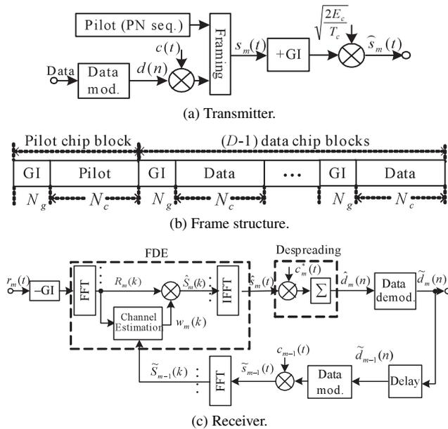
Fig. 1 DS-CDMA transmitter/receiver and frame structure.
