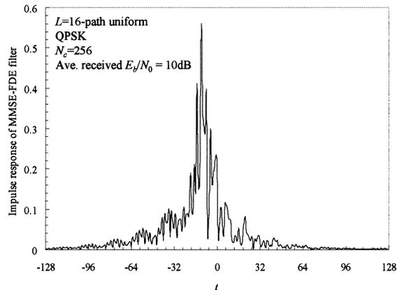
Fig. 2 Impulse response of MMSE-FDE filter.
