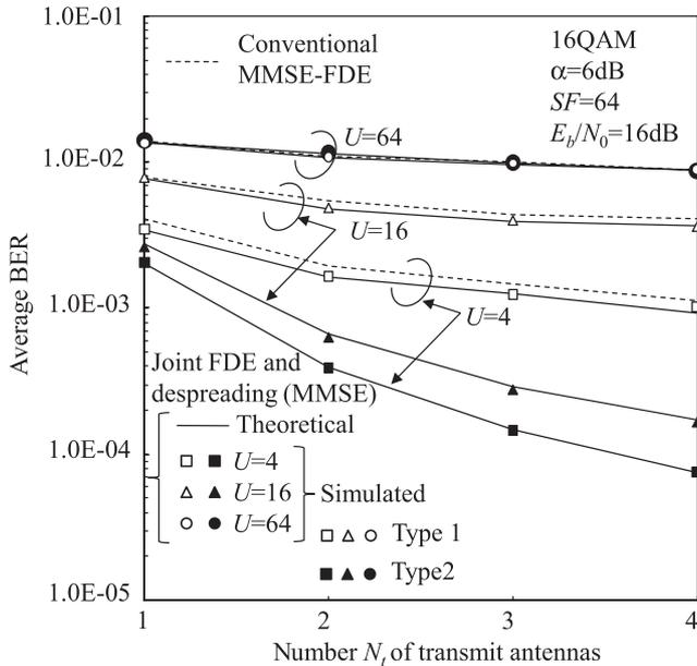
**Fig. 8** Impact of the number  $N_t$  of transmit antennas for multi-code transmission.
