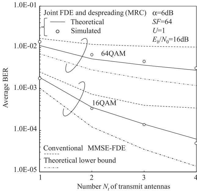
**Fig. 6** Impact of the number  $N_t$  of transmit antennas for single-code transmission.
