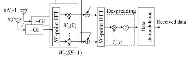
(a) Receiver structure of DS-CDMA using CDTD using the conventional MMSE-FDE.
