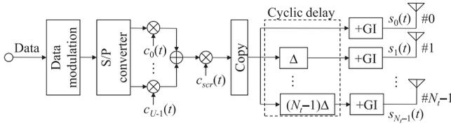
Fig. 1 Transmitter structure of multi-code DS-CDMA using CDTD.
