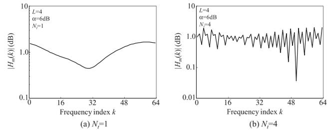
Fig. 3 Composite channel gain  $H_m(k)$  when  $\Delta = 16$ .
