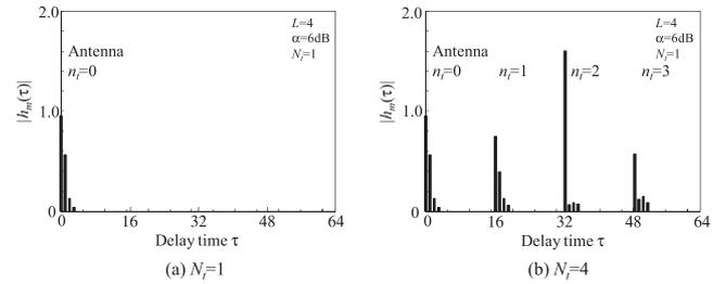
Fig. 2 Impulse response of the composite channel  $h_m(\tau)$  when  $\Delta = 16$ .
