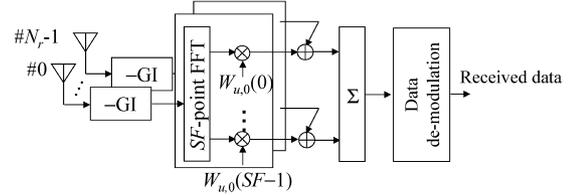
(b) Receiver structure of DS-CDMA using CDTD using the joint FDE and despreading.
