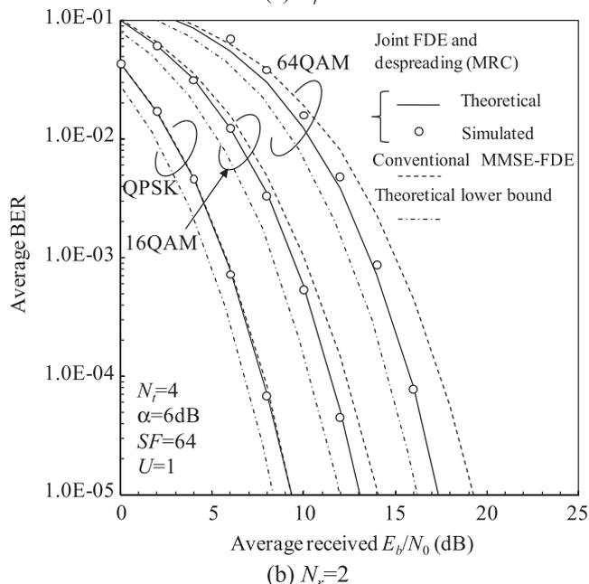
**Fig. 5** Theoretical and simulated BER performance with joint FDE and despreading for single-code transmission.
