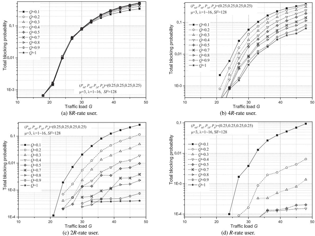
Fig. 11 Total blocking probabilities of different rate users.
