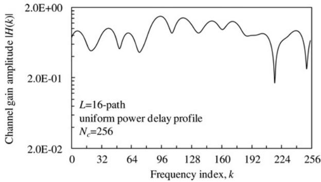
**Figure 2** One-shot observation of actual frequency-selective channel
