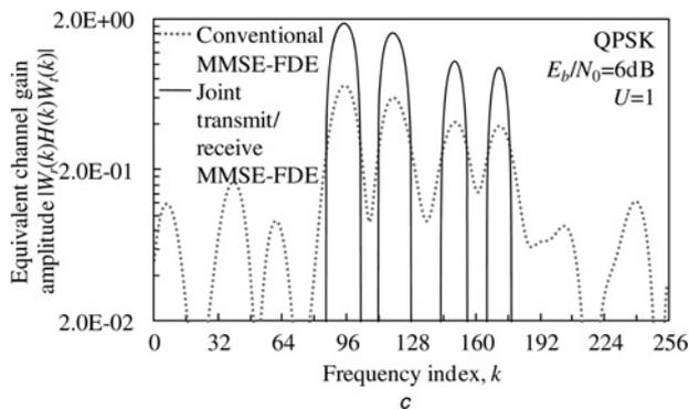
**Figure 3** Equivalent channel seen after the joint transmit/receive MMSE-FDE
