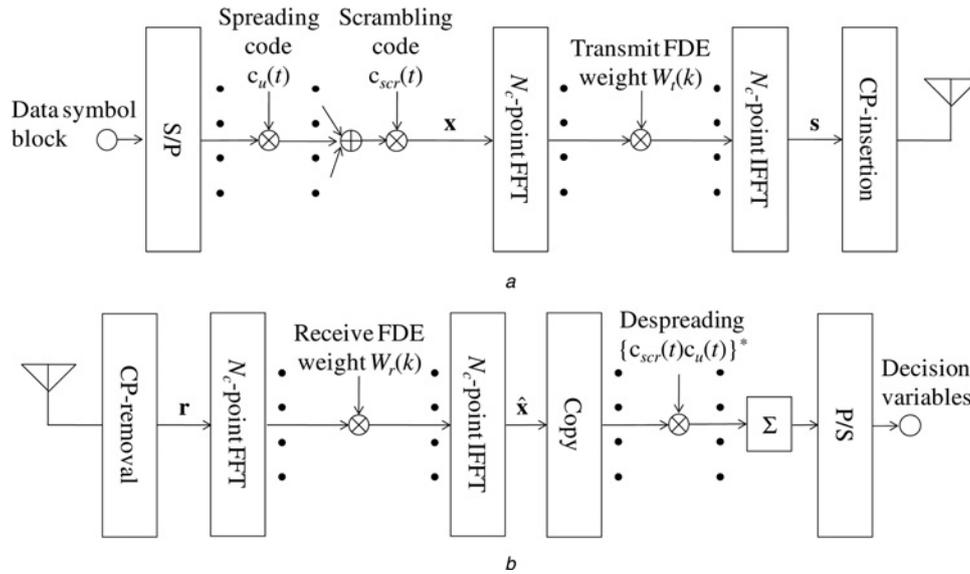
**Figure 1** Transmission system model of multicode DS-CDMA using proposed joint transmit/receive MMSE-FDE
