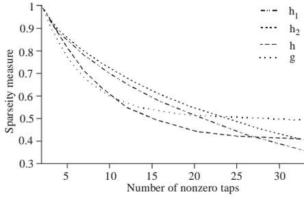
Fig. 1: Channel sparsity versus the number of nonzero channel taps
