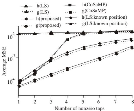
Fig. 3: MSE performance versus the number of nonzero channel taps (SNR = 10 dB)
