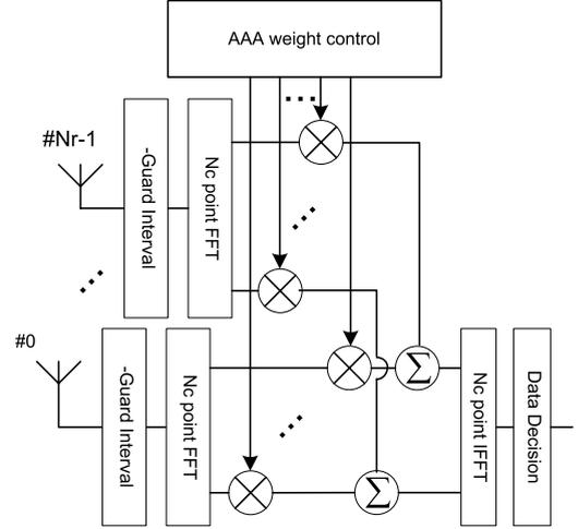
Fig. 4. Structure of FDAAA receiver.
