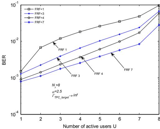
Fig. 7. BER performance of uplink SC multi-user MIMO detection,  $\alpha = 2.5$ .
