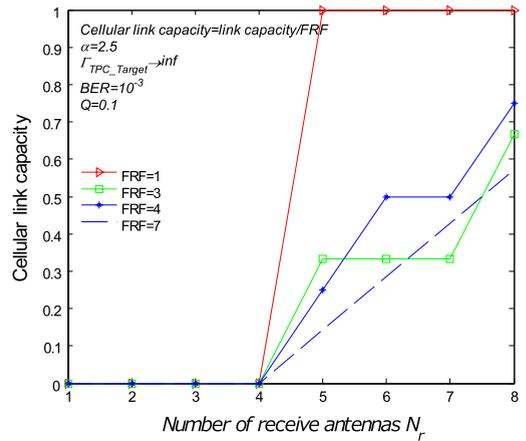
Fig. 11. Cellular link capacity,  $\alpha = 2.5$ .
