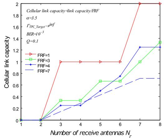
Fig. 12. Cellular link capacity,  $\alpha = 3.5$ .
