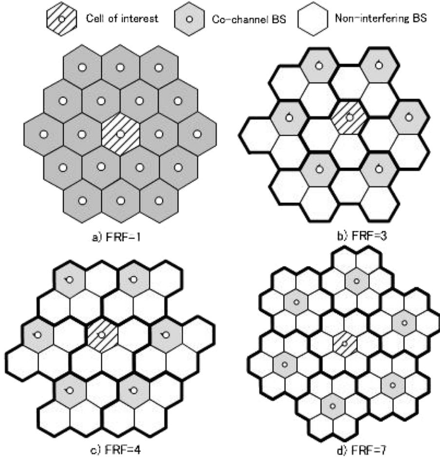
Fig. 2. Frequency reuse in cellular systems.
