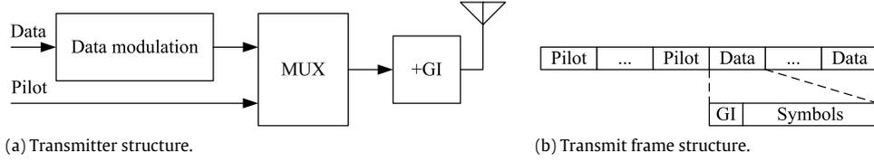
Fig. 3. Transmitter structure and transmit frame structure.
