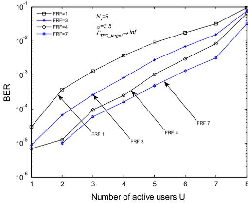
Fig. 8. BER performance of uplink SC multi-user MIMO detection,  $\alpha = 3.5$ .
