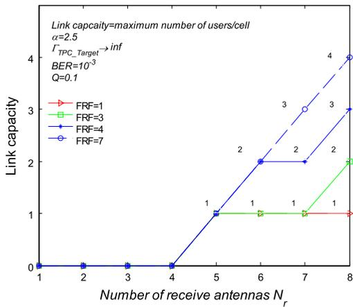
Fig. 9. Link capacity,  $\alpha = 2.5$ .
