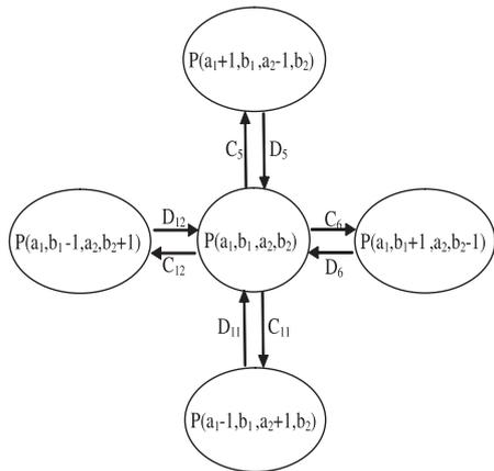
**Fig. 3** Possible handoff transitions from and to state  $P(a_1, b_1, a_2, b_2)$ .
