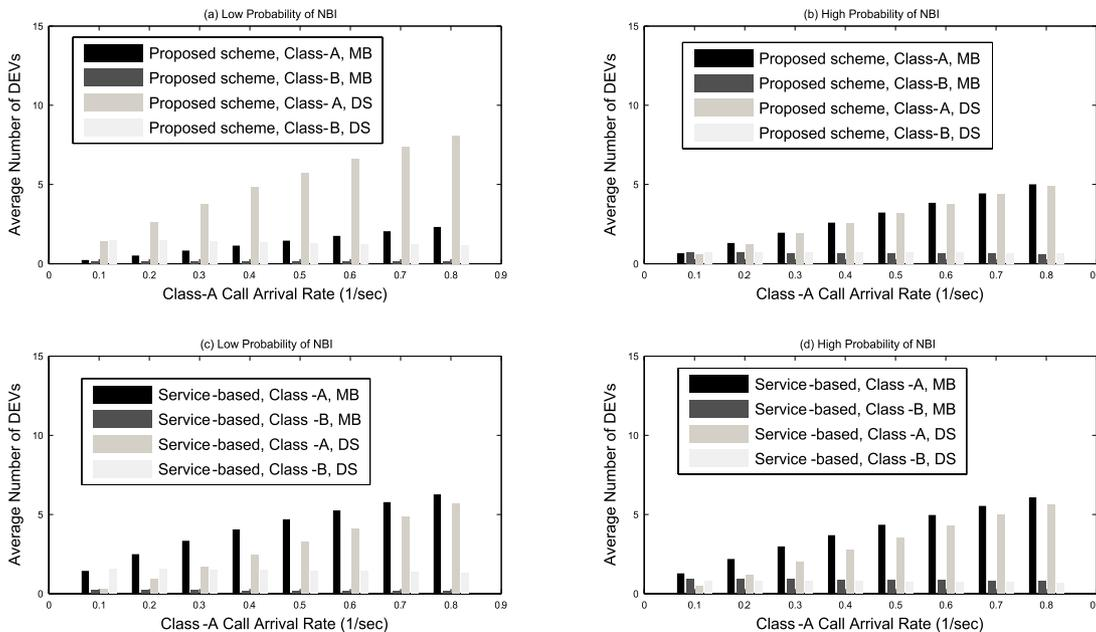
**Fig. 10** Average number of DEVs versus class-A call arrival rate for (a) the proposed scheme and low probability of NBI, (b) the proposed scheme and high probability of NBI, (c) the service-based scheme and low probability of NBI, and (d) the service-based scheme and higher probability of NBI.
