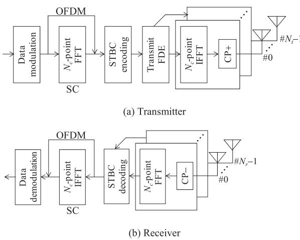
**Fig. 1** Transmitter/receiver structures.
