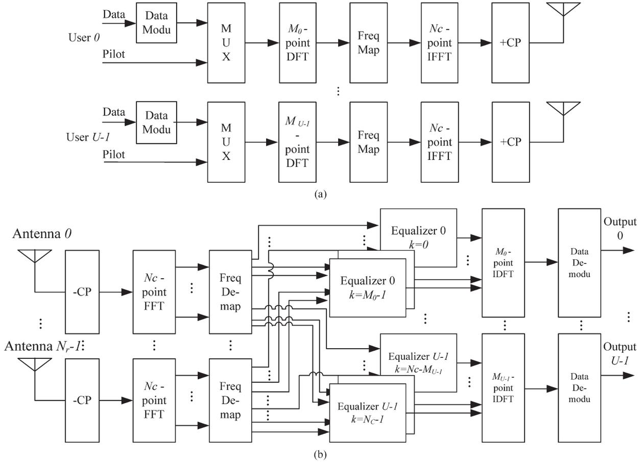
Fig. 3. Transceiver structure of SC-FDMA. (a) Transmitter structure. (b) Receiver structure.
