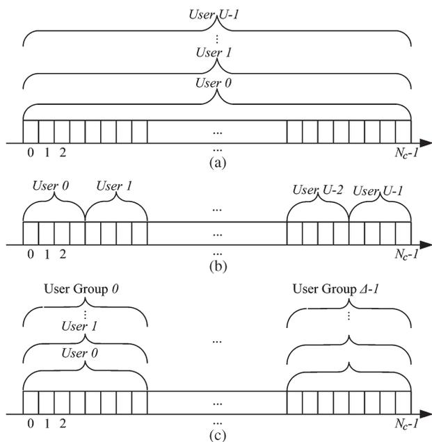
Fig. 6. Frequency allocation schemes of (a) SC-FDAAA, (b) SC-FDMA, and (c) SC-adaptive transceivers.
