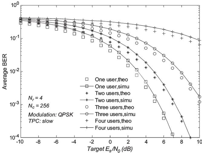
Fig. 7. Average BER performance of user 0; four-antenna SC-FDAAA receiver.
