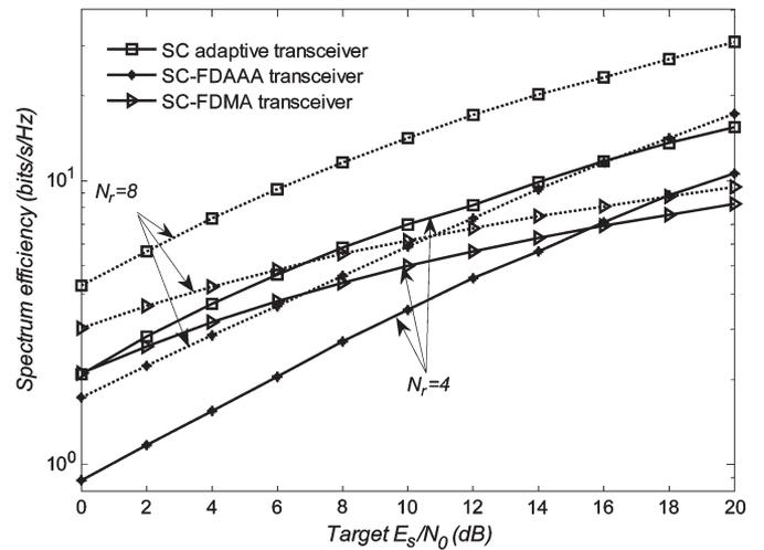
Fig. 9. Spectrum efficiency, SC multiuser MIMO with  $N_r = 4$  and  $N_r = 8$ .
