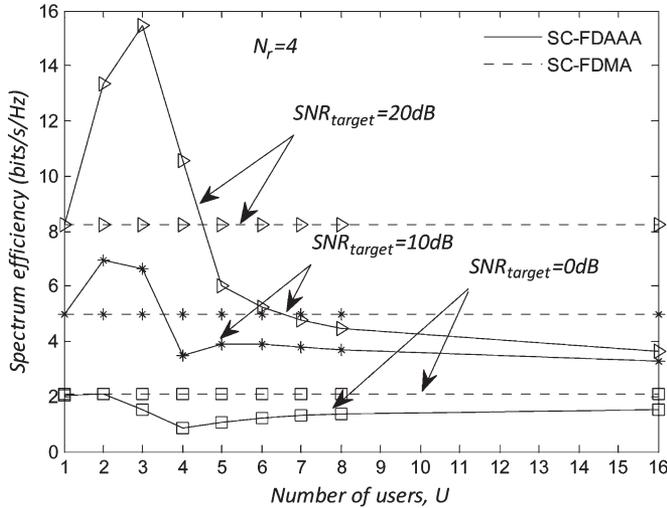
Fig. 4. Spectrum efficiency of a four-antenna multiuser SC MIMO system.
