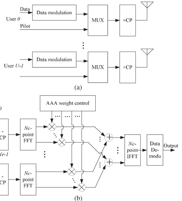
Fig. 2. Transceiver structure of SC-FDAAA. (a) Transmitter structure. (b) Receiver structure.
