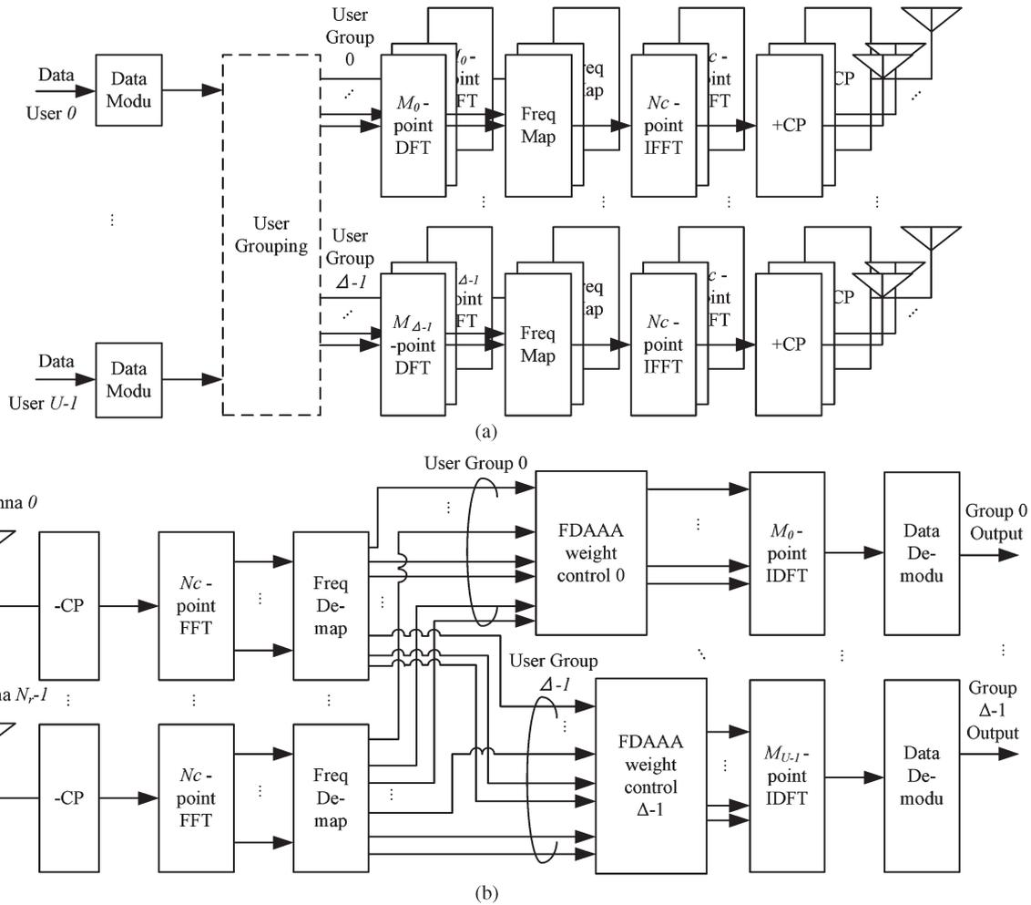
Fig. 5. SC-adaptive transceiver for multiuser MIMO system. (a) Transmitter structure. (b) Receiver structure.
