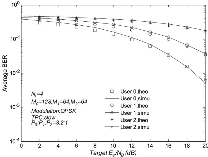
Fig. 8. Average BER performance for user 0, user 1, and user 2; SC-FDMA receiver.
