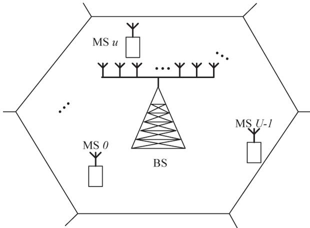
Fig. 1. SC uplink transmission in a single-cell multiuser MIMO system.
