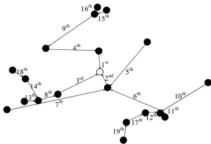
Fig.2 Model of the order of the links in the pre-assignment process of one VC.
