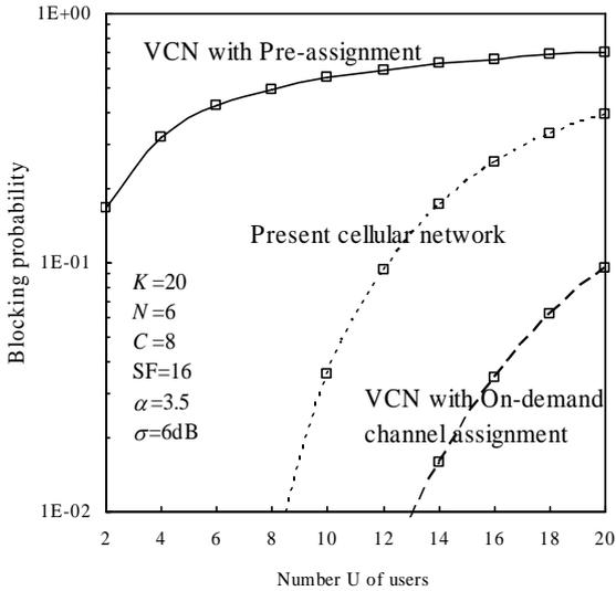
Fig.4 Blocking probabilities of the multi-hop VCN, using the pre-assignment and on-demand channel assignment, and the present cellular network.
