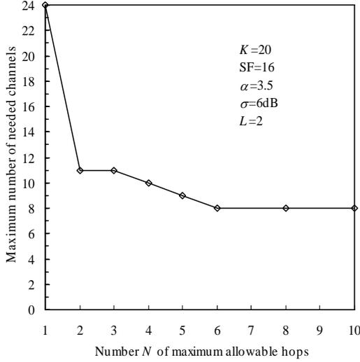
Fig.3 Maximum number  $C$  of channels needed for the pre-assignment of the multi-hop links between the WPs and the CP in one VC.
