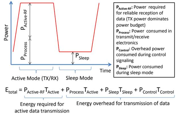
Fig. 4. Total wireless energy consumption at a BS.
