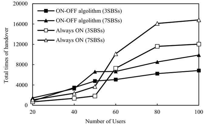
Fig. 6. Total number of HO vs different number of UEs is shown at an average velocity of 4km/h
