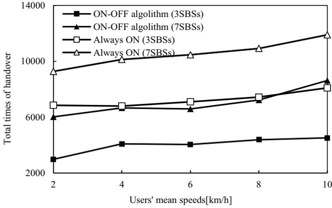
Fig. 3. Total number of HO vs different average velocities for 60 UEs and two different SBS numbers, i.e., 3 and 7
