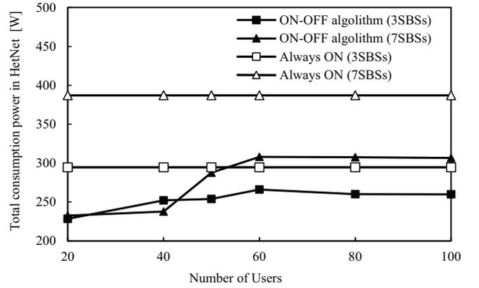
Fig. 5. The total consumption power in HetNet vs different number of UEs at an average velocity of 4km/h
