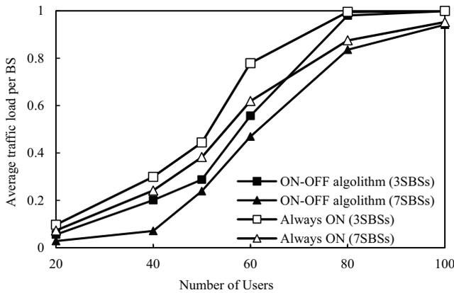
Fig. 4. The average traffic load per BS vs different number of UEs under the average velocity of 4km/h
